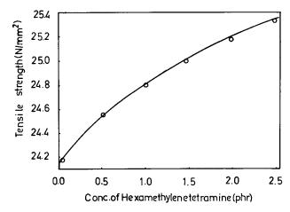
**Figure 5** Variation of tensile strength with concentration of hexamethylenetetramine in the rubber compound.
