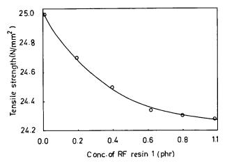
**Figure 8** Variation of tensile strength with concentration of RF resin I in the rubber compound.
