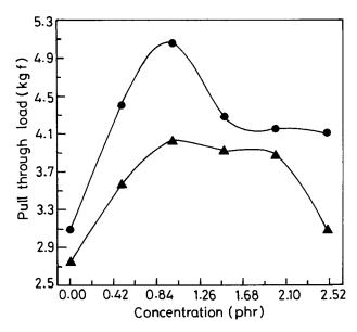
**Figure 3** Variation of pull-through load with hexamethylenetetramine in rubber compound. (●) NR latex/RF resin I-based RFL adhesive. (▲) NR latex/RF resin II-based RFL adhesive.
