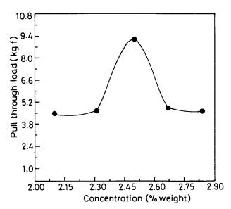
Figure 2 Variation of pull-through load with RF resin I to rubber ratio in VP latex-based RFL adhesive.
