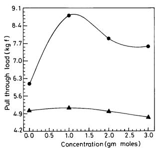
**Figure 6** Variation of pull-through load with donor (paraformaldehyde) in the RFL adhesive. (●) VP latex. (△) NR latex.
