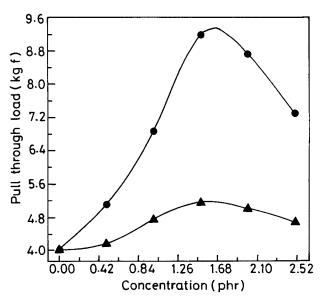
Figure 4 Variation of pull-through load with hexamethylenetetramine in rubber compound. (●) VP latex/RF resin I-based RFL adhesive. (▲) VP latex/RF resin II-based RFL adhesive.
