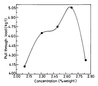
**Figure 1** Variation of pull-through load with RF resin I to rubber ratio in the NR latex-based RFL adhesive.
