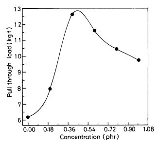
**Figure 7** Variation of pull-through load with donor (RF resin I) in the rubber compound.
